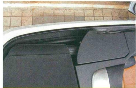
Folded roof doesn't fit flush with body; mechanism exposed.
